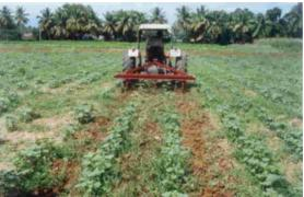
An inter cultivator cum earthing up equipment was developed and fitted to a standard tractor drawn ridger. Three number of sweep type blades are affixed to the ridger frame for accomplishing the weeding operation in between standing rows of crops. Three ridger bottom fitted behind the sweep blade, work on the loosened soil mass and aid in earthing up by forming ridges and furrows. Weeding efficiency is 61 per cent.
