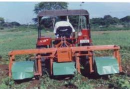
The multi row rotary weeder consists of a set of cutting blades, which penetrate in to the soil, removing the weeds in the crop rows. The cutting blade has also been used as an inclined plane for elevating and converging the soil. The rotating blades are used to cut the weeds and pulverizing the soil. Weeding efficiency is 71 per cent.
