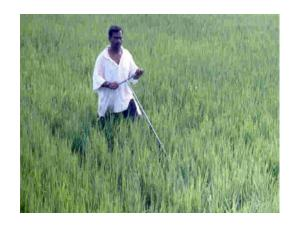
The cono weeder has two conical rotors mounted in tandem with opposite orientation. Smooth and serrated blades mounted alternately on the rotor uproot and burry weeds because the rotors create a back and forth movement in the top 3 cm of soil, the cono weeder can satisfactorily weed in a single forward pass without a push pull movement. It is easy to operate by a single operator. The weeder does not sink in puddled soil. Field capacity 0.18 ha/day. Star, Peg type and Twin hoe wheel weeding.
